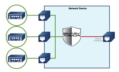
Virtual Network Appliance Installations insert Binary Armor cybersecurity into cutting edge OEM network equipment, including network switches, firewalls, and access points.
