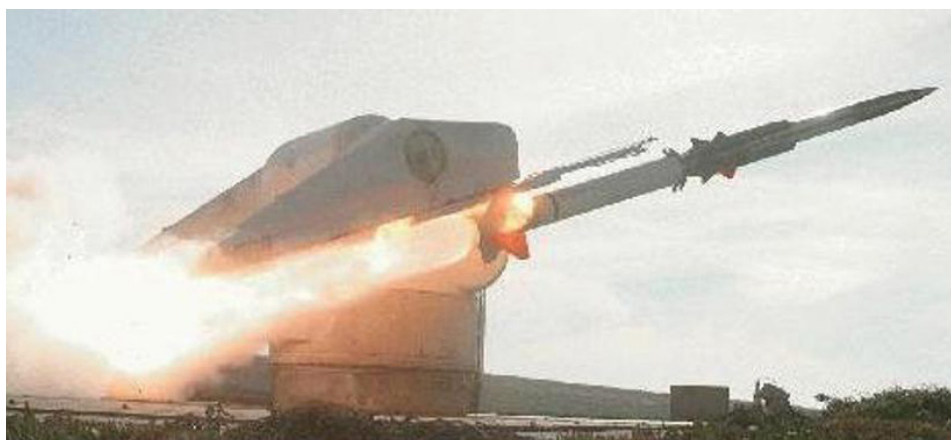
A GQM-163A SUPERSONIC SEA SKIMMING TARGET MISSILE FIRES FROM A SURFACE LAUNCHER. U.S. NAVY
