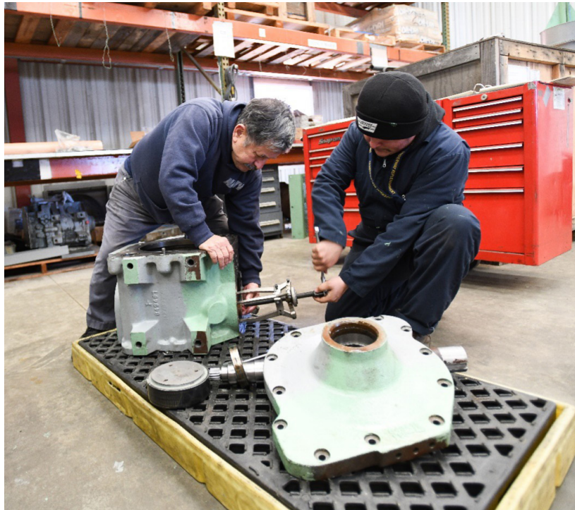
JOSE LEON (LEFT), SENIOR ENGINEERING TECHNICIAN, AND ALFREDO RUIZ, ENGINEERING TECHNICIAN, AT THE UNDERWAY REPLENISHMENT (UNREP) TEST SITE AT NSWC PHD, WORK TOGETHER TO REPAIR A HYDRAULIC PUMP ON MARCH 1. LEON FIRST RETIRED FROM THE NAVY IN 1991, AND REJOINED UNREP AS A CIVILIAN THE FOLLOWING YEAR. HE AGAIN RETIRED IN 2016 AND CAME BACK AGAIN IN 2018 TO SET UP A TRANSMISSION REBUILDING PROGRAM WITH YOUNGER CO-WORKERS LIKE RUIZ WHO NEED GUIDANCE. (U.S. NAVY PHOTO BY DANA RENE WHITE/RELEASED)
