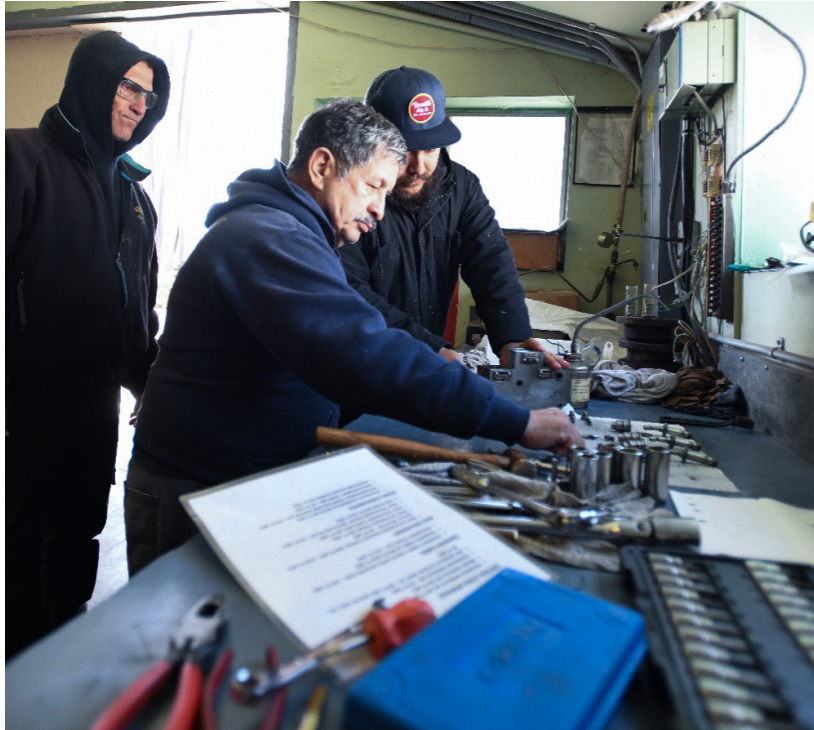
FROM LEFT: GIL NEGRETTE, ENGINEERING TECHNICIAN, JOSE LEON, SENIOR ENGINEERING TECHNICIAN, AND MARIO ESTRADA, ENGINEERING TECHNICIAN, HELP EACH OTHER REBUILD PART OF A HYDRAULIC TRANSMISSION AT THE UNDERWAY REPLENISHMENT TRANSMISSION REFURBISHMENT SHOP AT NSWC PHD ON MARCH 1. LEON RETURNED FROM A SECOND RETIREMENT TO HELP YOUNGER TECHNICIANS KEEP THE FLEET COMBAT READY. (U.S. NAVY PHOTO BY DANA RENE WHITE/RELEASED)
