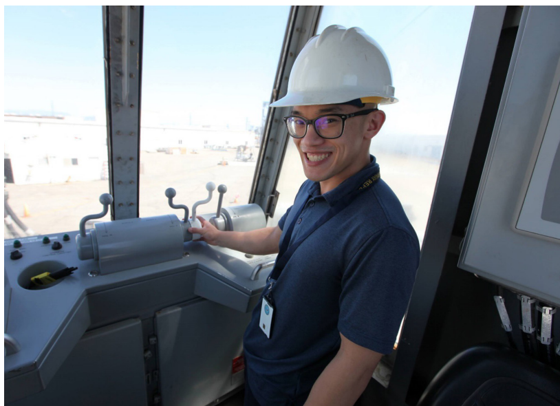
NSWC PHD UNDERWAY REPLENISHMENT (UNREP) MECHANICAL ENGINEER BRYAN NGUYEN DEMONSTRATES HOW A PROTOTYPE SADDLE HANDLE (IN WHITE), WHICH HE CREATED USING A 3D PRINTER, HAS BEEN FLIPPED 180 DEGREES FROM ITS ORIGINAL POSITION SO THAT IT NOW LIES CLOSER TO THE STRAIGHT SADDLE HANDLE TO ITS RIGHT, THUS ALLOWING AN UNREP OPERATOR TO CONTROL BOTH HANDLES SIMULTANEOUSLY WITH ONE HAND. THE SADDLE HANDLES, LOCATED AT THE COMMAND’S UNREP TEST SITE, ARE USED TO CONTROL FUEL LINES. (U.S. NAVY PHOTO BY TERI CARNICELLI/RELEASED)
