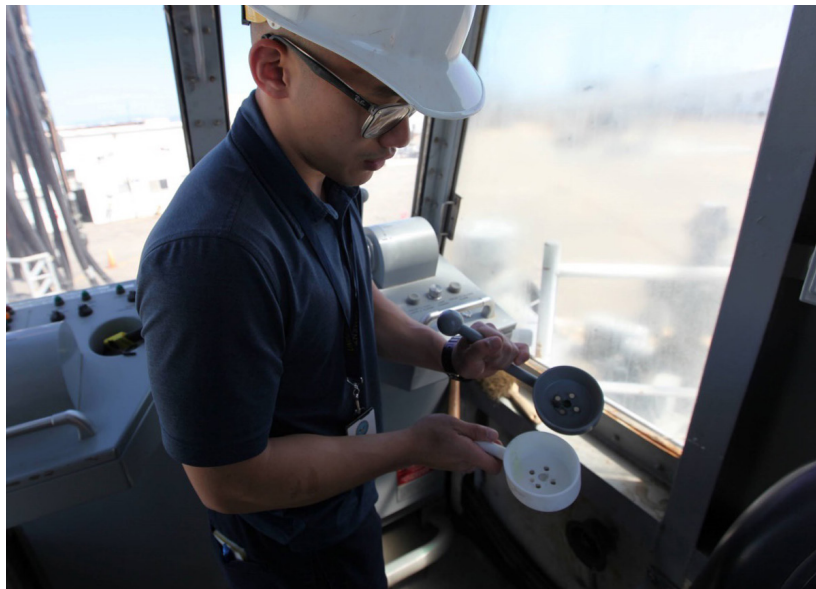
UNREP MECHANICAL ENGINEER BRYAN NGUYEN SHOWS OFF TWO OF FOUR PROTOTYPE SADDLE HANDLES USED TO CONTROL FUEL LINES DURING AN UNDERWAY REPLENISHMENT (UNREP). NGUYEN USED THE PLASTIC 3D PRINTER AT THE COMMAND’S OFFSITE FATHOMWERX LAB TO ENGINEER THE HANDLES THAT CONTAIN THREE COMPONENTS: THE ROUND KNOB AT THE TOP, THE STEM AND THE CUP-SHAPED BASE. THE WHITE HANDLE PROVED TO BE TOO CLOSE TO THE ADJACENT SADDLE HANDLE, SO NGUYEN DESIGNED ANOTHER ONE (IN BLACK) WITH A SHORTER OFFSET TO ADD SPACE BACK BETWEEN THE TWO HANDLES. (U.S. NAVY PHOTO BY TERI CARNICELLI/RELEASED)
