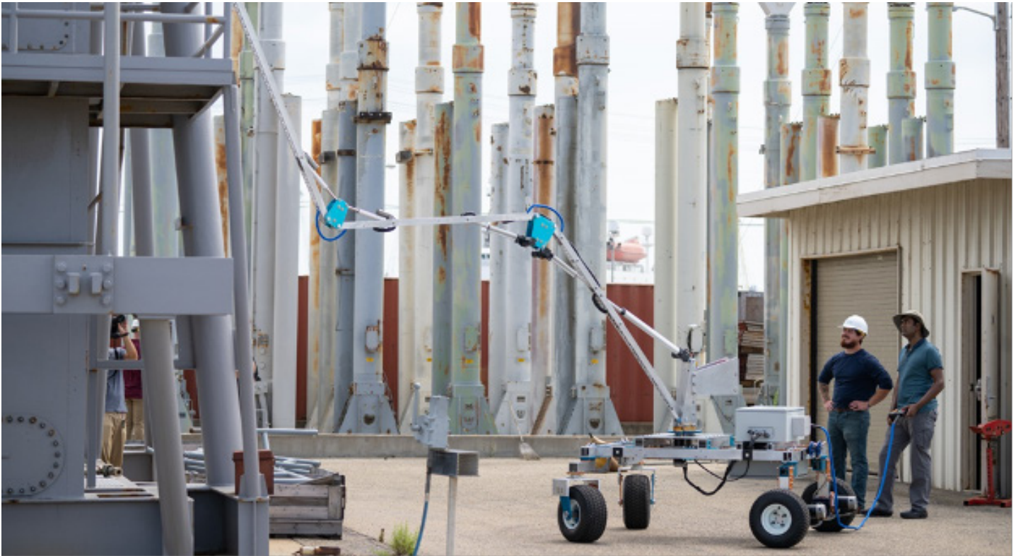
FROM LEFT: AROBOTICS CO. MACHINIST MIKE BONDRA AND CHIEF EXECUTIVE OFFICER AKAASH KANCHARLA WATCH THE WHEELED NDTEST-R ROBOT EXTEND ITS ARM TO THE UPPER LEVELS OF A STRUCTURE AT NSWC PHD'S UNDERWAY REPLENISHMENT TEST SITE ON SEPT. 11 AS PART OF THE 2023 COASTAL TRIDENT SERIES ADVANCED NAVAL TECHNOLOGY EXERCISES. (U.S. NAVY PHOTO BY ERIC PARSONS/RELEASED)
