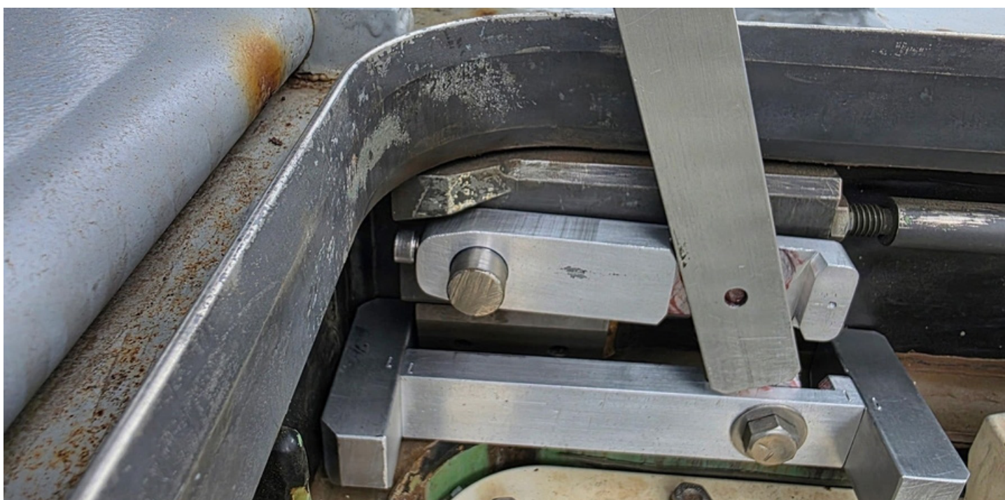
PHOTO PROVIDED BY ERIC CSORBA. AN EARLIER VERSION OF A PROTOTYPE TOOL THAT NAVAL SURFACE WARFARE CENTER, PORT HUENEME DIVISION (NSWC PHD) ENGINEERING TECHNICIAN ERIC CSORBA DESIGNED ENGAGES A LATCH ROD INSIDE A MK 41 VERTICAL LAUNCHING SYSTEM (VLS) CELL AT NSWC PHD'S LAUNCHER LAB IN PORT HUENEME, CALIFORNIA, ON JUNE 4. TESTING CONFIRMED THAT THE TOOL ACTUATES THE LATCH ROD WITHOUT DAMAGING THE CELL MOUTH OR COMPROMISING THE HATCH SEAL.
