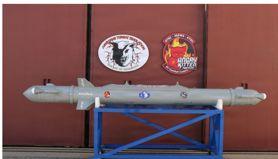
PHOTO BY KIMBERLY BROWN | AN ANGRY KITTEN ELECTRONIC WARFARE POD SITS ON A MAINTENANCE STAND AT NAVAL AIR WARFARE CENTER WEAPONS DIVISION. NAWCWD ENGINEERS INTEGRATED AND MATURED THE POD SYSTEM THROUGH A PARTNERSHIP WITH GEORGIA TECH RESEARCH INSTITUTE, GIVING WARFIGHTERS A GOVERNMENT-OWNED JAMMER CAPABLE OF SUPPRESSING ENEMY AIR DEFENSES.
